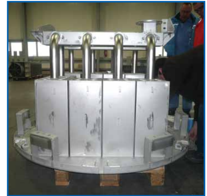
The cyclones deck fitted to the top of the cage
