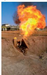
A burn pit is an area devoted to open-air combustion of hydrocarbons. In Qatar, there are many gas fields with several burn pits to combust the excess gas released during start-up, shut down and emergency situations. The Dukhan gas fields in Qatar comprise eight burn pits. To adhere to the environmental and safety objectives set in place, the burn pits are replaced by elevated flare systems (60 metres tall) with a smokeless combustion.
